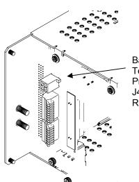
Battery Temperature Probe Connector J410 (Rear Cover Removed)
